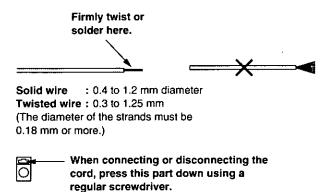
Failure to twist the end of the cord firmly can cause short-circuiting.
