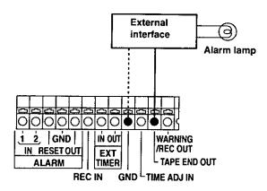
When the cassette tape comes to its end during recording, the alarm device which has been installed externally is triggered.
