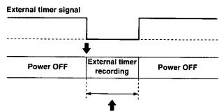
Recording proceeds in the recording mode which was set by menu screen P4 RECORDING MODE.
