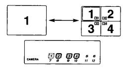
Four camera numbers are enclosed in squares on the camera number display of the display tube, and the square corresponding to the number of the selected camera flashes. In addition, the numbers of the cameras (C01/C02/C03/C04) appear in the center of the TV monitor.
