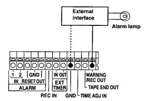
The auto OFF output and recording output connections are the same. Select between them using ERROR WARN/REC OUT on the menu screen shown on P7 TERMINAL OUTPUT SELECT.
