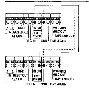
When using a second time lapse recorder as the external switch for setting the time
