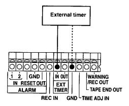
An external timer can be used for recording.
