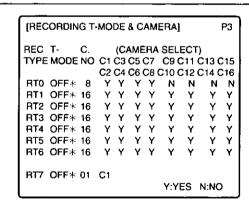
When recording always in the same recording time mode instead of setting the mode using the TIME MODE button, set RT1 through RT7 for the REC TYPE item on the setting menu shown on the P3 RECORDING T-MODE & CAMERA screen, and set the REC TYPE (RT1 through RT7) to be used for recording for the REC-TYPE item on the P4 RECORDING MODE screen.
